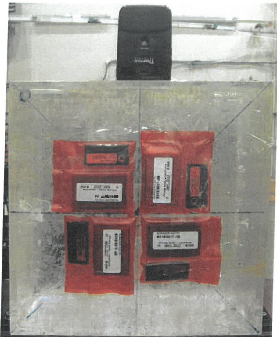
*Figure 1: Rotationally symmetric arrangement employed for the irradiations of groups of four dosimeters.*
